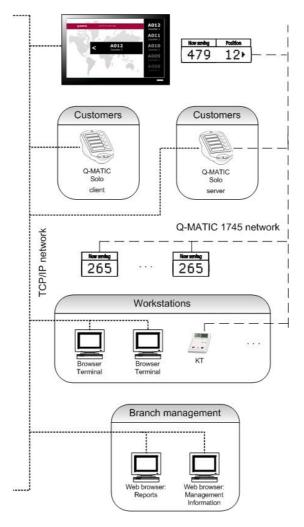
This is a schematic picture of a large Qmatic Solo System.
